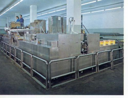
A packaging system developed by Nicolaus, Kempten, for the Union Brewery in Dortmund, Germany. Both machine and special pack for ten bottles were designed for fully automatic operation.
